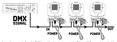
**CAUTION!** At the last unit, you must close the DMX line with a terminating resistor. Take an XLR connector and solder a 120 0hm resistor between signal (-) and signal (+) and connect it to the DMX output of the last unit in the line.
